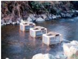
Equipment for sampling stream-spawning kokanee fry as they outmigrate the spawning channel into Mission Creek and Okanagan Lake. The data is used to estimate the productivity of the channel.
